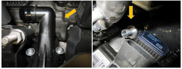
**19**. Fit the silicone hose from the oil breather adaptor on the head to the barbed fitting on the silicone elbow.
