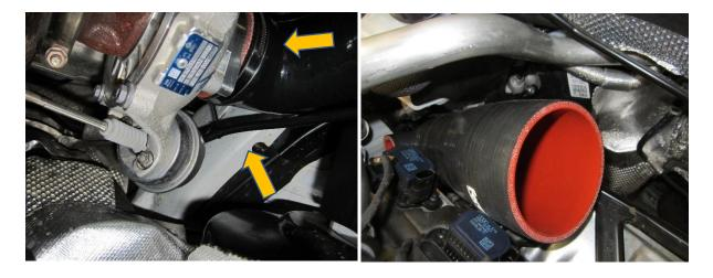
**18**. Refit the oil breather adaptor to the head and fit the barbed fitting supplied into the silicone elbow.
