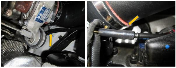
**16**. Remove the plastic pipe from the oil breather adaptor by either heating with a heat gun or by using a sharp knife to cut.
