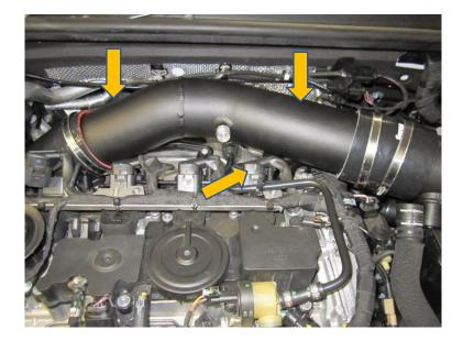
21. Pull the silicone hose up onto the hard pipe and tighten the hose clamp.
