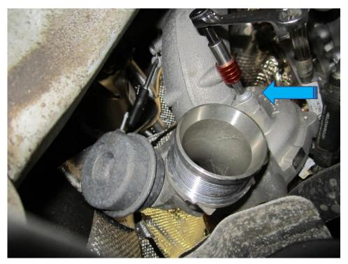
14. Fit the new turbo adaptor into position ensuring the supplied O-ring is fitted in the ring groove of the adaptor. Please note if you are fitting the FMINLH9 TTE625/700 the O-ring is not supplied as this is situated on the mounting face of the turbo.
