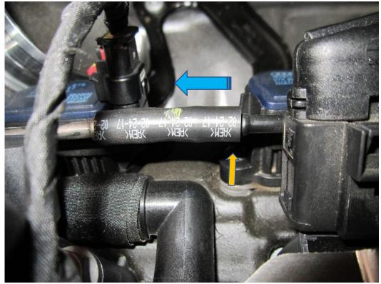
12. Using a 10mm socket and suitable drive undo the nuts that hold the coil packs in position, then using a T20 Torx drive remove the oil breather adaptor pictured below.
