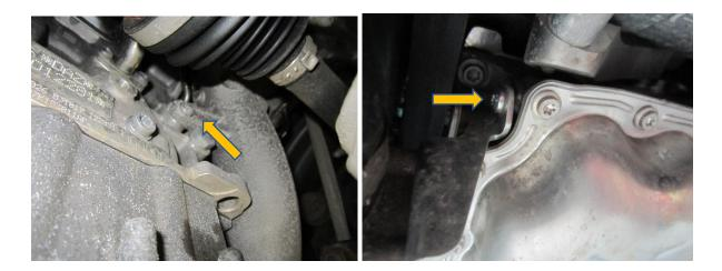
8. Undo the hose clamps that are still holding the boost pipe in situ.
