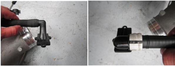
17. Fit the silicone hose to the turbo adaptor and fit the hose clamp into position ensuring it is pushed fully onto the adaptor and the hose clamp is tightened between the swage of the adaptor and the base.
