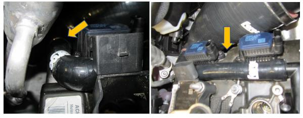
20. Fit the Forge Motorsport FMINLH8 turbo intake pipe making sure the M6 X 25 bolt and penny washer are securely in place.
